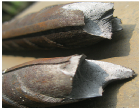
Incomplete Cup-cone fracture (necking found, i.e. Ductile)
