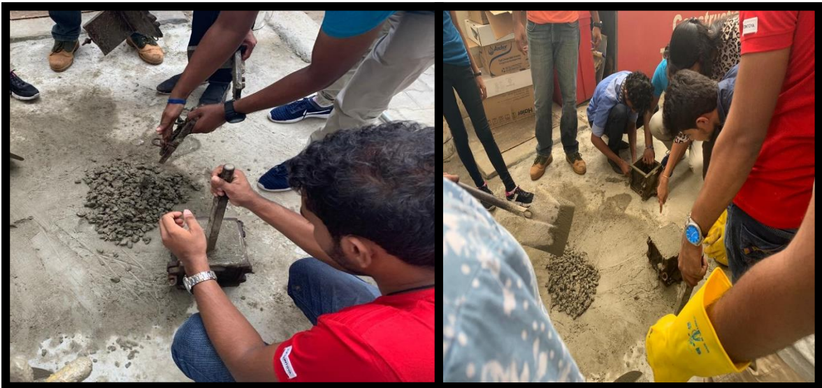
Figure 9 - How the group members were filled the cubes and compacted each layer 35 times using the steel rod
