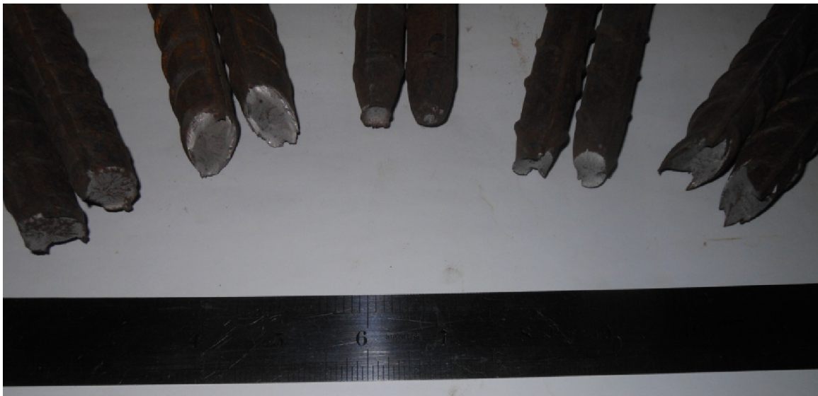
Incomplete Cup-cone fracture (necking found, i.e. Ductile)
