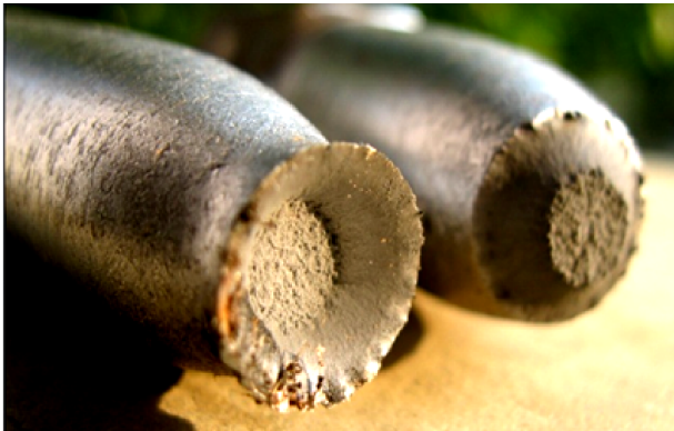
Cup-cone fracture (necking found, i.e. Ductile)
