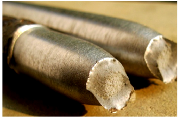
Incomplete Cup-cone fracture (necking found, i.e. Ductile)
