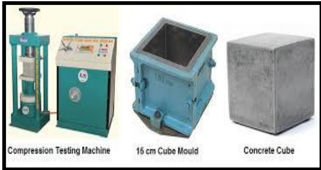
Figure 1 - Concrete Cube Test kit set (Anon., n.d.)
