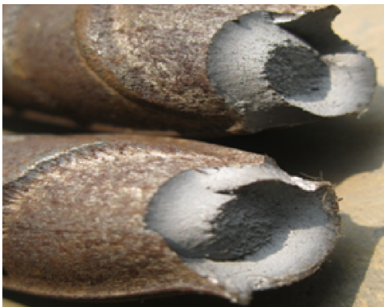
Incomplete Cup-cone fracture (necking found, i.e. Ductile)
